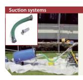
With the HeavyCoat piston pumps material can be applied directly from a 120 litre drum or from large containers.
