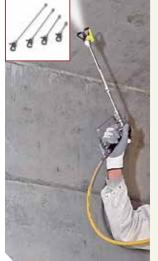
The use of nozzle extensions saves using ladders and scaffolding, extends the radius of action for objects with large surfaces and thus increases working flexibility.
